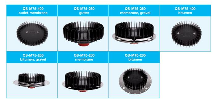
The Wavin range of metal roof outlets are easy to install and maintain, with only 2 screws per outlet and no special tools required. The "260" outlets have a high nominal maximum flow rate; the "400" outlets have the same flow rate for a lower water level on the roof. This means fewer of the "400" outlets are needed to drain the same volume of water (approx 30% less
