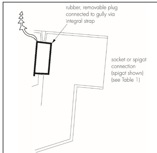
1.2 The outlet of the 6UR590 and 6UR600 gullies is suitable for connection to Osma 150 mm UltraRib pipe. The outlet of the 6TW650 and 6TW651 gullies is suitable for connection to Wavin 150 mm TwinWall spigot.
