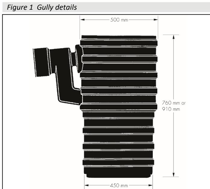
**Figure 2 Trap detail**
