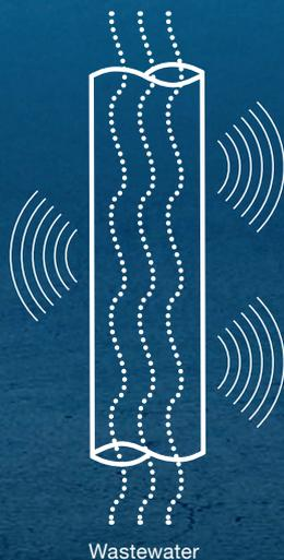
**Airborne sound** is the amount of noise from water passing through a pipe that can be heard if standing in the same room in which the pipe is installed
