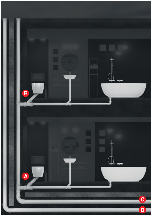
Fig. 11: Minimum fall for waste water pipes, example.
