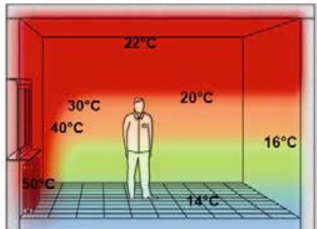
Air movement and heat distribution in the radiator system
