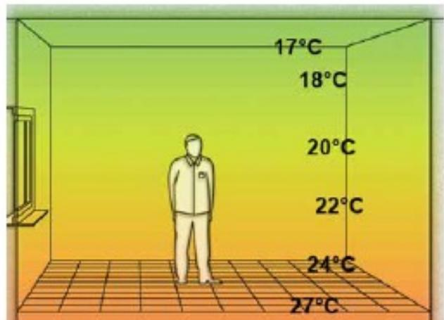
Air movement and heat distribution in the underfloor heating
