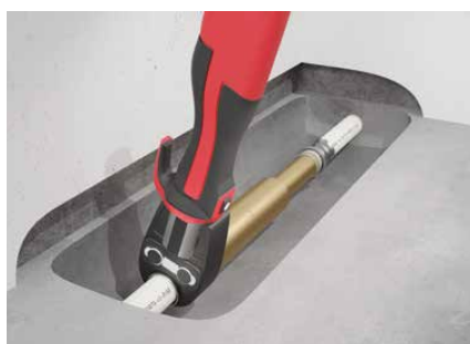
Fig. 29: Installationstrin, reparationskobling.
