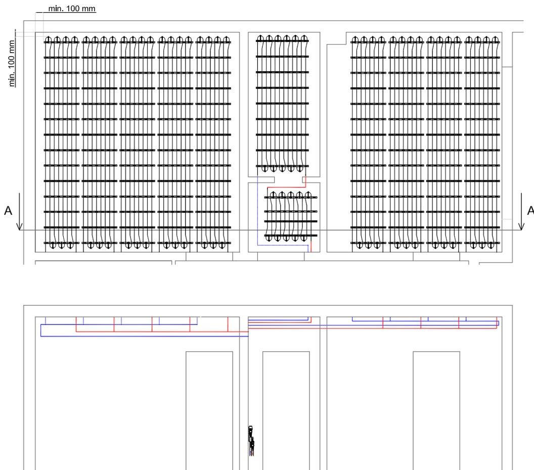
Fig. 1 Example of distribution for WW-10 ceiling panels
