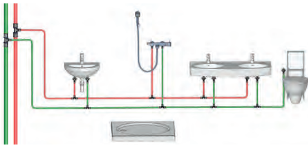
Example 1: Traditional distribution system, using individual Tee fittings to connect to each tap.
