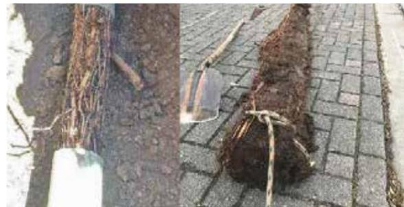
Pipe with standard gasket which has roots in it.
