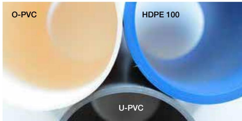
Wall thicknesses of different types of pipes with the same pressure strength
