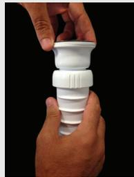
4- Connect the sink strainer to the upper union inlet part of the HepvO diaphragm by rotating it clockwise. Torque the gasket by tightening the union. The gasket that comes with the kit for d32 HepvO connection must be used separately.
