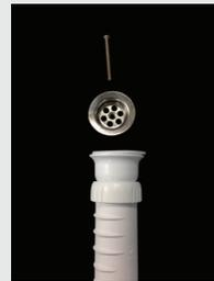
5- In order to connect it to the sink, remove the screw on top of the strainer and connect it so that the sink remains in between the metal strainer and the plastic base.
