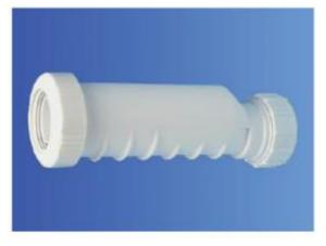
$Hep_VO^{\circledast}$  is a self-sealing waste valve for use as an alternative to a traditional water seal trap, in particular where a water seal trap is not suitable, for example, due to climate, movement of the appliance or because of infrequent use. Its in-line design and the option of either horizontal or vertical installation can save space. The valve can also reduce the requirement for additional venting of some appliances.
