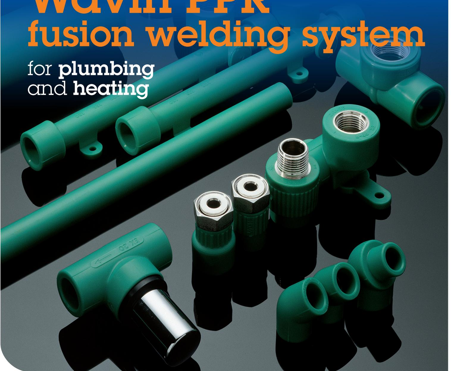
Wavin PPR is a hot and cold water supply system suitable for sanitary and potable water applications and heating systems. The pipes and injection moulded fittings are made of Polypropylene Random (PPR) type 3, also with new high performance pipes in PP-RCT (PP type 4). They are jointed by fusion welding, ensuring a homogeneous, all plastic system.
