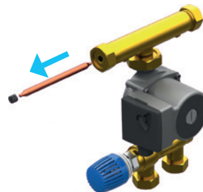
Figure 12: Remove flow water temperature sensor
